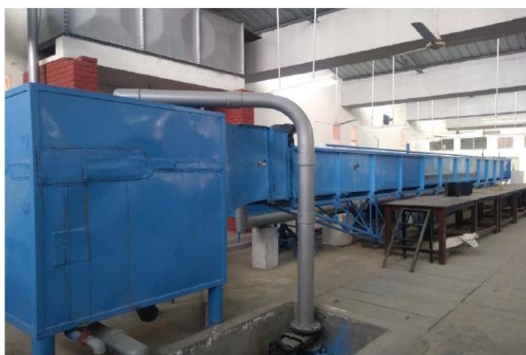
Figure 1. Tilting bed flume used in the experiment
