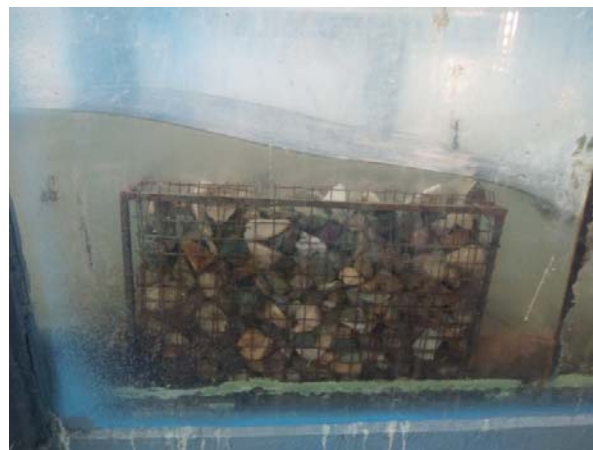
Figure2. Gabion weir used in the experiment
